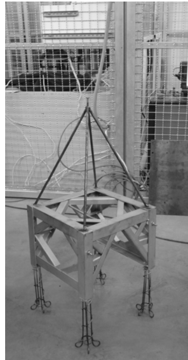
Fig. 4 Physical pole model designed to bury in homogeneous ground.
