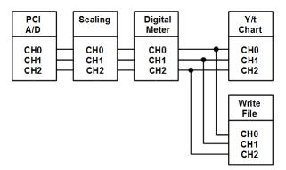
Fig. 2. Block diagram of the system for registering and visualising the time curves of voltage, current and rotational speed of the AC drive
