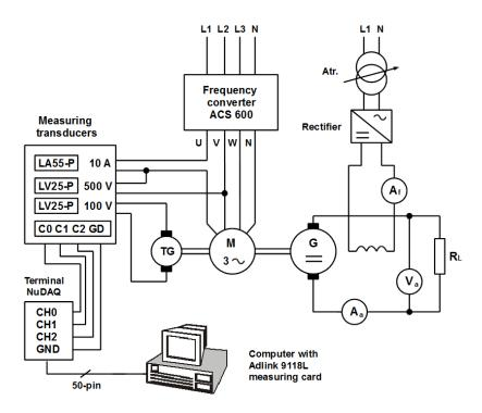
Fig. 1. Diagram representing connections in the AC frequency converter drive and the computer-based measuring system
