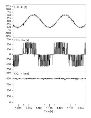
Fig. 4. Time characteristics of the phase current, phase-to-phase voltage and rotational speed for steady-state conditions
