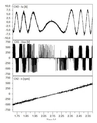
Fig. 5. Time characteristics of the phase current, phase-to-phase voltage and rotational speed at the reverse of the drive system
