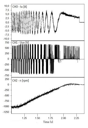
Fig. 6. Time characteristics of the phase current, phase-to-phase voltage and rotational speed at deceleration of the drive system
