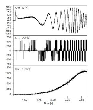
Fig. 3. Time characteristics of the phase current, phase-to-phase voltage and rotational speed at start-up
