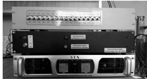
Fig. 14. Multiplexer, VCCS and power amp in 2U
