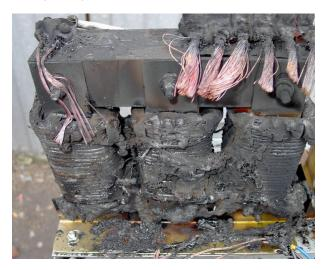
Fig. 5. Photograph of the choke of a passive filter damaged due to an overload caused by the incorrect design of the filter parameters
