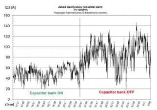
Fig. 4. Graph of a selected voltage harmonic measured at point A with a capacitor bank on and off
