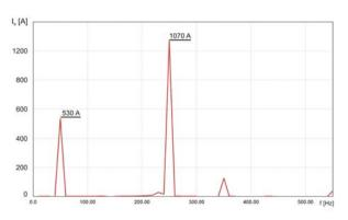
Fig. 14. Simulation of the 1st and 5th harmonic currents in a wornout capacitor bank
