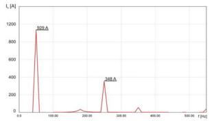
Fig. 13. Simulation of the  $\mathbf{1}^{st}$  and  $\mathbf{5}^{th}$  harmonic currents in a new capacitor bank
