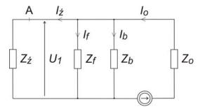
where:  $Z_{z}$  – power source impedance,  $Z_{r}$  – filter impedance,  $Z_{b}$  – capacitor bank impedance,  $Z_{o}$  – current source impedance.
