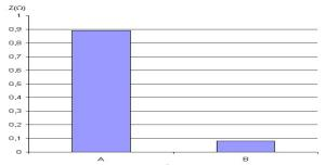
Fig. 12. Comparison graph of  $\mathbf{5}^{th}$  harmonic impedance of a new (A) and worn-out (B) step of a capacitor bank
