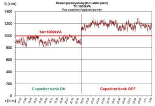
Fig. 3. Apparent power graph with a reactive power compensation unit correspondingly off and on
