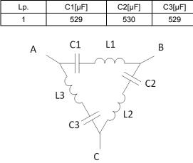
Fig. 8. Connection diagram of the tested capacitor bank and the choke
