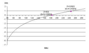
Fig. 9. Z (f) parameter for a 80kvar (400V) step of a brand-new capacitor bank
