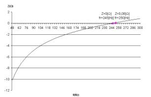
Fig. 11. Z(f) parameter for a 80kvar (400V) step of an old capacitor bank
