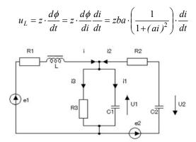
Fig. 7. The electrical circuit with a nonlinear coil [15]
