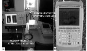
Fig.4. Spectrum analyzers used during calibration. a) RSA5106A RT Tektronix spectrum analyzer; b) FSH4 R&S handheld spectrum analyzer
