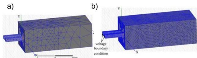
Fig. 5. Two analysed discretization meshes: (a) coarse mesh, (b) dense mesh
