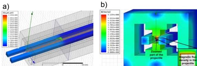
Fig.6. Calculation results for  $U_c=200$  V: (a) the current density distribution in the rails and projectile, (b) magnetic flux density distribution
