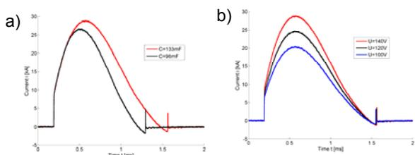
Fig.10. Current excitation waves for different supply parameters: (a) constant voltage value ( $U_c=141$  V) - different capacity values; (b) constant capacitance value ( $C=133$  mF) - variable voltage values
