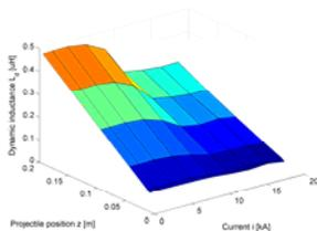
Fig.8. Dynamic inductance vs. current value and projectile position
