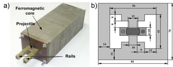
Fig.1. Electrodynamic accelerator with ferromagnetic core (ICR), (a) picture of the prototype, (b) cross-section (dimensions in mm)
