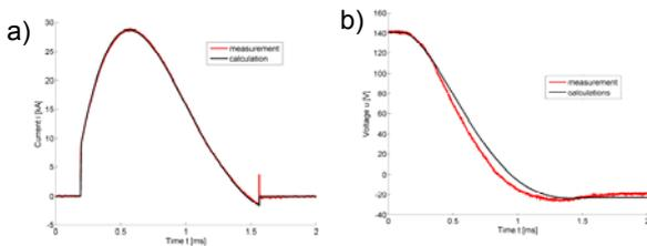
Fig.11. Measurement verification of the field-circuit model for  $U_c=141$  V and  $C=133$  mF: (a) excitation current wave; (b) voltage wave
