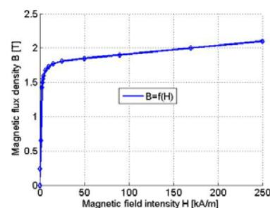
Fig.2. Measured B/H curve of the used ferromagnetic core
