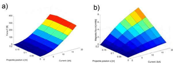
Fig.7. Calculations of the integral quantities vs. projectile position and excitation current value: (a) electrodynamic force, (b) magnetic flux
