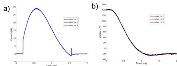
Fig.9. Repeatability tests for  $U_c=141$  V and  $C=133$  mF: (a) current excitation waves; (b) voltage waves
