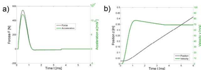
Fig.12. Calculated waves for  $U_c=141$  V and  $C=133$  mF: (a) force and acceleration; (b) position and velocity
