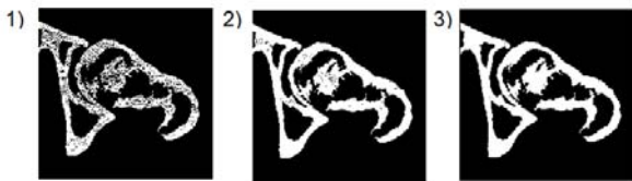
Fig.7. Segmentation result after 200 iterations with the number of ants equal to: 1) 15% 2) 30% 3) 50% of the pixels number in the image
