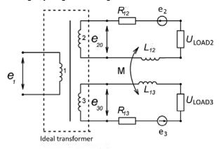
Fig.3. Equivalent circuit of a three-winding transformer
