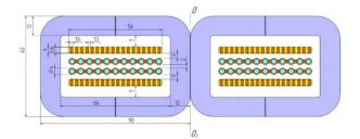
Fig.10. The new design of the transformer for RSW system
