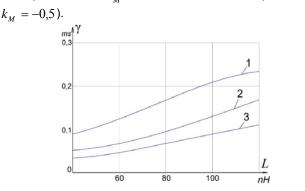
Fig.7. The switching time  $\gamma$  vs the leakage inductance *L* at a frequency of 1 kHz
