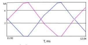
Fig.9. Currents  $i_2$  ,  $i_3$  vs time in the secondary windings at f=10 kHz
