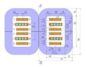
Fig.2. Design of the basic transformer TR1.
