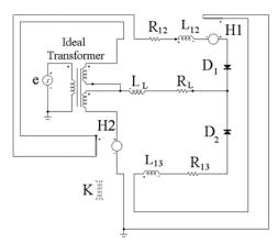
Fig.5. The model for RSW system simulation
