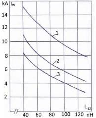
Fig.6. The influence of the leakage inductance on the RMS welding current (curve 1 corresponds to  $k_M$ =0.5, curve 2 corresponds to  $k_M$ =0, curve 3 corresponds to  $k_M$ =0.5)
