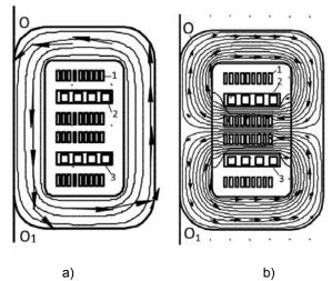
Fig.4. The magnetic fluxes of the transformer 1-2 a) open circuit (main flux), b) short circuit (leakage flux)
