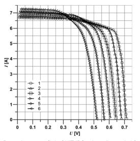
Fig.6. Dependences I = f(U) of HIT-IBC solar cell recorded for  $E = 1000 \text{ W/m}^2$  and different operating temperatures  $T_p$ : 1 – 253 K, 2 – 273 K, 3 – 298 K, 4 – 323 K, 5 – 348 K, 6 – 373 K
