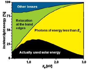
Fig.1. Distribution of the energy losses in solar cell, presented as the dependency of the incident light percentage in the function of band gap value  $E_g$  [9]
