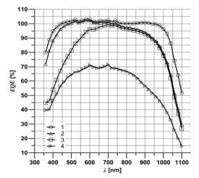
Fig.2. Dependences  $EQE = f(\lambda)$  for different types of c-Si solar cells: 1 – HIT-IBC, 2 – EWT, 3 – HIT, 4 – conventional cell
