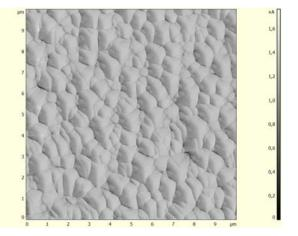
Fig.4. SEM micrograph showing the front surface of the examined HIT-IBC solar cell
