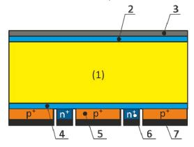
Fig.3. Schematic diagram of the tested HIT-IBC solar cell structure (sample 1): 1 - n-type silicon substrate, 2 - front passivation layer, 3 - anti-reflective coating, 4 - a-Si intrinsic thin layer,  $5 - p^+$  - type region,  $6 - n^+$  - type region, 7 - electrode
