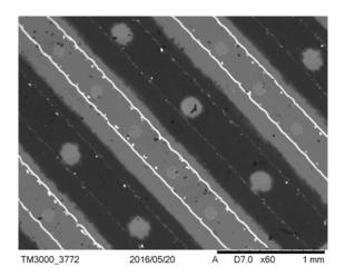
Fig.5. SEM micrograph showing the rear surface of the examined HIT-IBC solar cell
