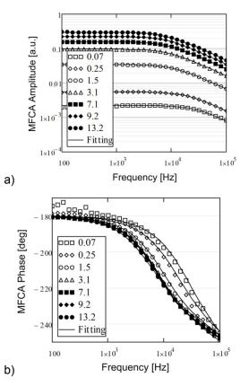
Fig.2. a) MFCA amplitude signal and b) MFCA phase signal characteristics, obtained for different levels of excitation (from *I*=0.07 to 13.2 W/cm<sup>2</sup>) and the wavelength of the illuminating light  $\lambda$ =808 [nm]. Solid lines represent theoretical lines, symbols are experimental data
