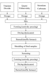
Fig. 3. Technological scheme for production of prototypes
