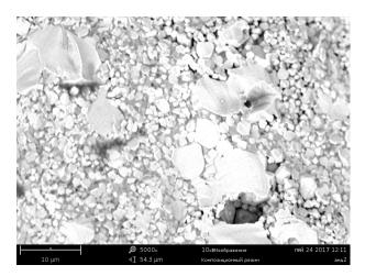
Fig. 5. Microstructure of the ceramics of the composition "II" (firing temperature 1330  $^{\circ}\text{C})$
