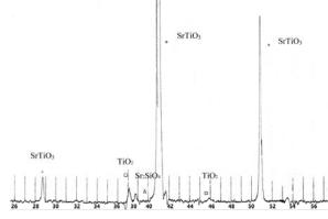
Fig. 4. Bar-radiograph of the sample "II" (firing temperature 1,330  $^\circ\text{C})$
