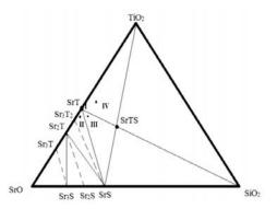
Fig. 2. Diagram of the state of the three-component system SrO -TiO<sub>2</sub> – SiO<sub>2</sub> [15]
