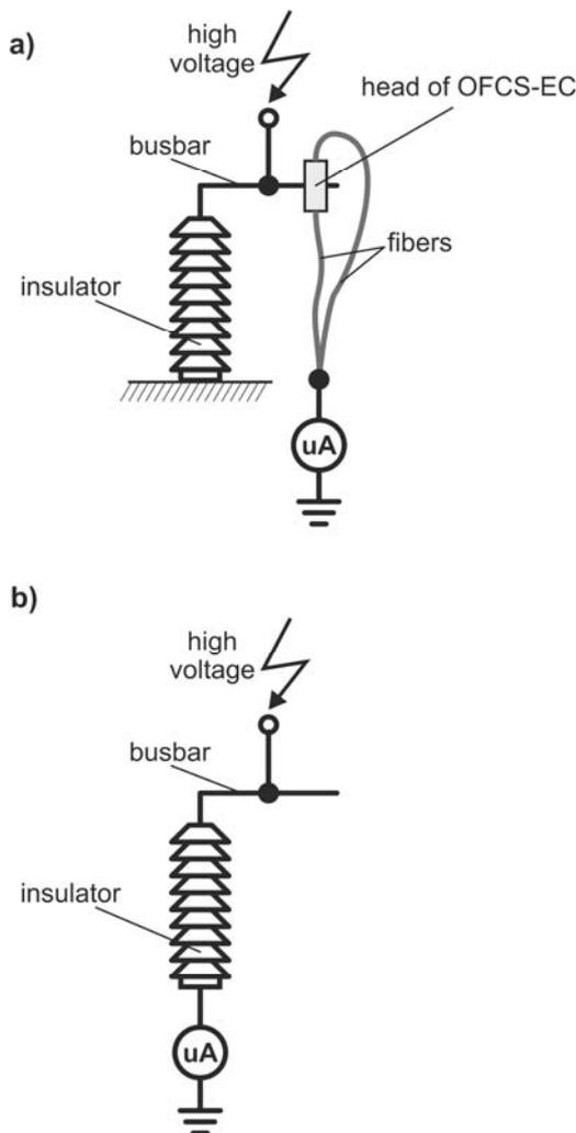
Fig. 2. Schematic view of setup for leakage current measurements: a) OFCS-EC sensor, b) supporting insulator
