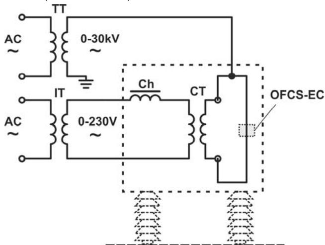
Fig.4. Electrical scheme of a setup used for tests under high voltage and current conditions. (TT – test transformer; IT – insulating transformer; Ch – choke; CT – current transformer)
