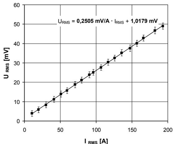
Fig.6. The response of the sensor as a function of electric current intensity in busbar for voltage 30 kV
