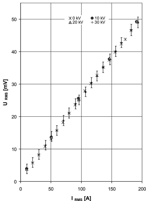
Fig.7. Collective plot of sensor's response registered for the following values of voltage: 0 kV, 10 kV, 20 kV and 30 kV
