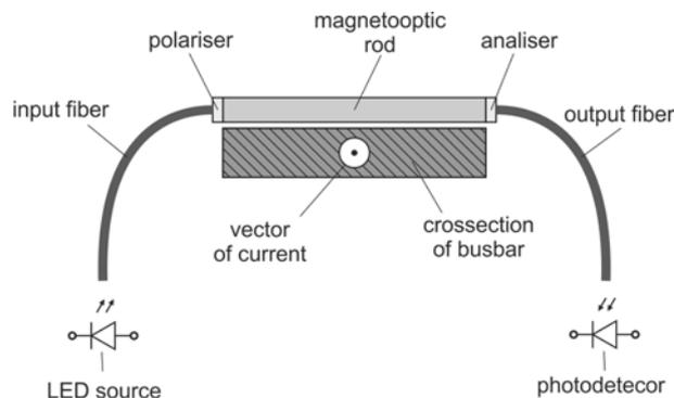
Fig.1. A schematic drawing of the optical fiber current sensor with external conversion investigated in this paper
