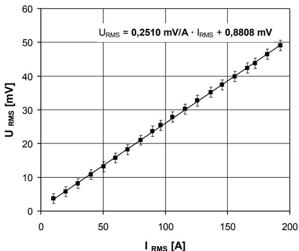
Fig.5. The response of the sensor as a function of electric current intensity in busbar for voltage 0 kV
