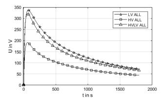
Fig.4. RV-curves measurements on TR2 ( $U_p$  = 1 kV,  $t_p$  = 1800 s)
