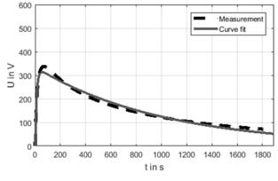
Fig.7. Curve fit for TR2 at LV ALL with 2 elements
