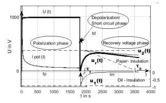
Fig.1. Basic principle of the measurements according to PCRV
