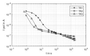
Fig.2. Polarization current Ip for 3 units at 1 kV (LV-All setup)
