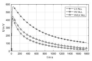
Fig .5. RV-curves measurements on TR3 ( $U_p$  = 1 kV,  $t_p$  = 1800 s)
