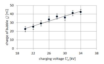
Fig.9. The charge of single soap bubble  ${\it Q}$  as a function of charging voltage  $U_{\rm e}$
