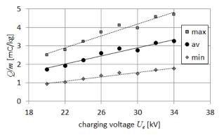
Fig.10. Parameter (Q/m) of single soap bubble as a function of charging voltage  $U_e$  for extremes and average mass values. "max" = maximum (Q/m) value calculated for minimal mass  $m_b$  = 9 mg, "av" - average (Q/m) value, "min" = minimum (Q/m) value for maximum mass  $m_b$  = 24 mg
