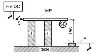
Fig.3. Scheme of setup for soap bubble observation. SB – soap bubble, S – mechanical switch, MP – metal pipe, HV DC – DC high voltage supply, I – insulating supports, E – grounded electrode
