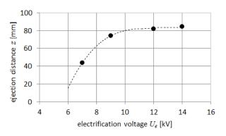
Fig.7. Ejection distance z as a function of applied voltage  $U_e$
