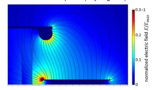
Fig.4. Normalized (to maximum value) electric field distribution and electric field lines just after HV application (soap bubble is undeformed)
