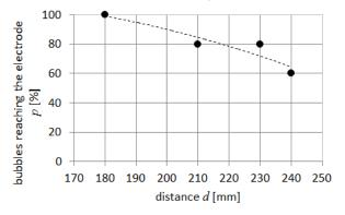
Fig.12. Percentage of bubbles p reaching the electrode as a function of distance  $\boldsymbol{d}$
