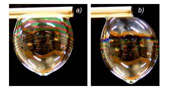
Fig.5. Same soap bubble a) without an electric field, b) after applying 6 kV voltage on the metal pipe
