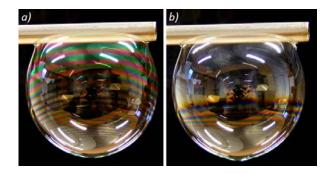
Fig.2. Observation of water film drainage on a single soap bubble: a) bubble about 20 s after blowing (time needed to prepare camera settings), b) bubble after additional 5 s, just before bursting
