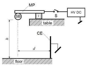
Fig.11. Setup for observing charged bubbles trajectory, CE – collecting electrode, h = 800 mm
