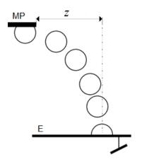
Fig.6. Soap bubble falling off from metal pipe – image based on images from the recorded film using a digital camera. z – ejection distance
