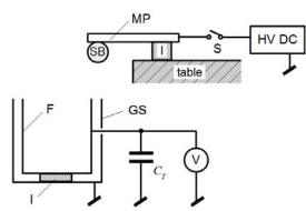
Fig.8. Setup for soap bubble charge measurement, GS – grounded shield, F – Faraday cup, SB – soap bubble, S – mechanical switch, MP – metal pipe, HV DC – DC high voltage supply, I – insulating supports
