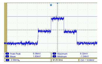
Fig.5. Current consuption profile for BME280 sensor
