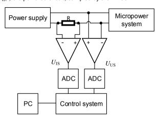
Fig. 1. Energy measurement method implementation using energy definition
