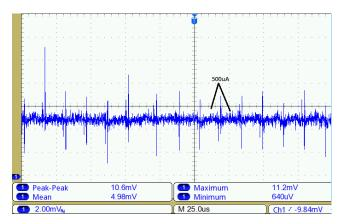
Fig.8. Current consuption profile for MSP432P401R normal run
