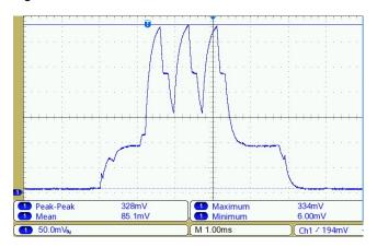
Fig.9. Current consuption profile for HC-08 Bluetooth module working in energy-saving MODE1 and 4 dBm output power during data transmission
