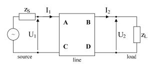
Fig.3. Simplified model of power supply line as a long line
