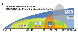
Fig.1. Frequency ranges dedicated for PLC transmission in compliance with EN 50065
