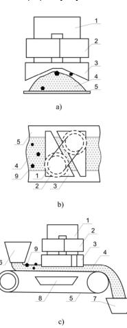
Fig. 1. Suspended electromagnetic iron separator with arch-shaped pole pieces (a – view along the conveyor belt; b – top view; c – overview), where 1 – magnetic system; 2 – magnetizing coil; 3 – pole piece; 4 – separated material; 5 – conveyor belt; 6 – initial material bunker; 7 – purified material bunker, 8 – bunker for the extracted ferromagnetic bodies; 9 – ferromagnetic bodies
