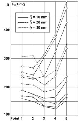
Fig. 3. Experimental curves representing the distribution of the force field across the width of the suspended iron separator working zone at the depth of extraction
