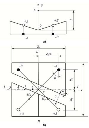
Fig. 2. Calculated model of the inter-pole work space (a – front view; b – top view)
