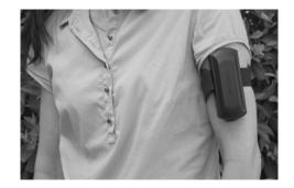
Fig. 2. An image of one of the ESM 140 dosimeters used in the tests together with the method of its installation
