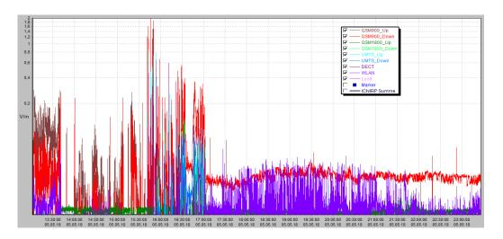
Fig. 3. E intensity values of the electromagnetic field measured in two locations. Measurements from 1.00 to 4.00 p.m. in the area of Stryjów, one hour trip by car, from 5.00 p.m. staying on an estate in Orłów Murowany.
