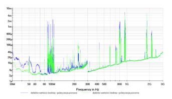
Fig. 1. Electromagnetic spectrum in the range 30MHz-3GHz on a scale from  $\mu V/m$  to mV/m in the town of Bełżec, measurement 10.05.2018
