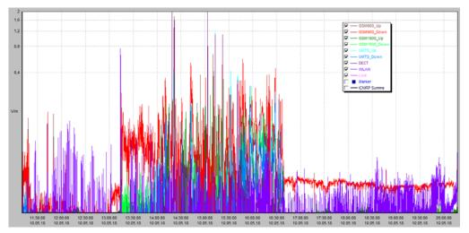
Fig. 4. The values of the intensity E of the electromagnetic field measured on the Lublin-Bełżec route (until 1.00 p.m.), on the premises of a single-family house by 4.30 and on the way back.
