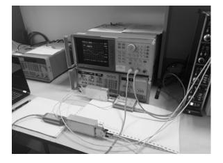
Fig.2. Laboratory test stand for the determination of the frequency and transfer characteristics.
