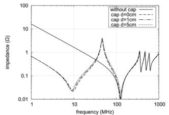
Fig. 4. PDN impedance for different distances between IC and decoupling capacitor (four layers stackup with 5 mils between planes).
