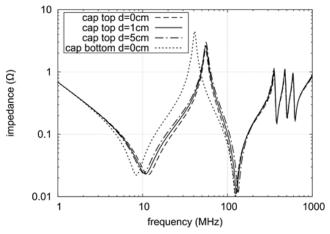
Fig. 12. PDN impedance for different capacitor placement (8-layer stackup, blind via).
