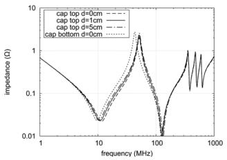
Fig. 11. PDN impedance for different capacitor placement (8-layer stackup, through via).
