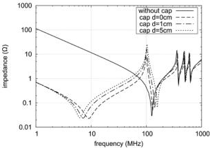
Fig. 3. PDN impedance for different distances between IC and decoupling capacitor (four layers stackup with 35 mils between planes).
