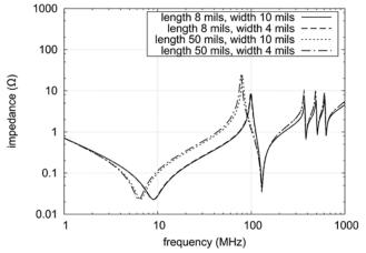
Fig. 5. PDN impedance for different capacitor mounting (capacitor close to the IC, four layers stackup with 35 mils between planes).
