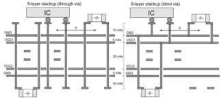
Fig. 10. Capacitor placement for 8-layer stackup.
