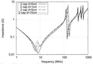
Fig. 6. PDN impedance for different distances between IC and second decoupling capacitor (one capacitor close to the IC, four layers stackup with 35 mils between planes).
