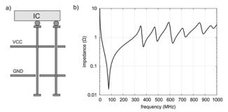
Fig. 1. A 4-layer stackup (a) and frequency behaviour of power planes (b).
