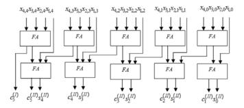
Fig.3. 5-bit 4-operand CSA adder
