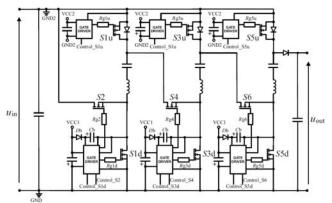
Fig.5. The proposed gate driver system in the SYSCVM
