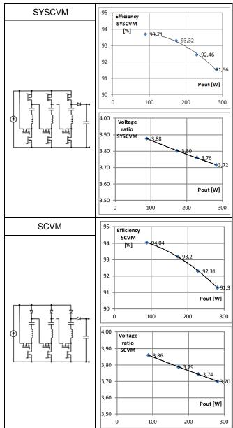
Fig.8. Experimental results of the SYSCVM. Results of measurements of efficiency and the voltage ratio versus power of the SYSCVM and SCVM converters.  $U_{in} = 30V$
