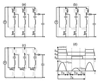
Fig.2. Operating principle of the SYSCVM: (a) charging of the capacitors through the lower and upper MOSFET transistors, (b) charging of the capacitors through the lower transistors and upper diodes, (c) discharging of the capacitors, (d) control of switches and parameters of waveforms
