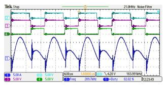
Fig.6. Experimental results of the SYSCVM. Waveforms of the input current (1) and control signals of groups of transistors: lower charging transistors (2), upper charging transistors (3), discharging transistors (4).  $U_{in}$  = 40 V,  $P_{out}$  = 200 W
