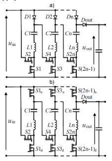
Fig.1. DC-DC converter in the topology of: (a) basic Resonant Switched-Capacitor Voltage Multiplier (SCVM), (b) Synchronous Resonant Switched-Capacitor Voltage Multiplier (SYSCVM) [9]
