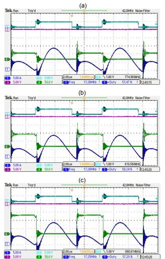
Fig.7. Experimental results of the SYSCVM. Waveforms of the input current (1) and voltage on the upper switch (4): the  $S_{1u}$  (a), the  $S_{2u}$  (b), the  $S_{3u}$  (c).  $U_{in}$  = 40V. Channel (2) displays control signal of lower charging transistors
