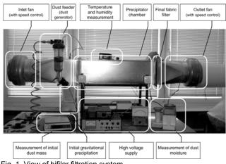
Fig. 1. View of bifilar filtration system
