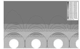
Fig. 4. Distribution of electric field intensity in bifilar winding with a solid chassis (voltage 10 kV, wire cross-section 1.0  $\rm mm^2)$
