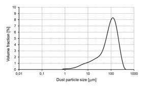
Fig. 2c. Volume distribution of dust particle size for C type dust
