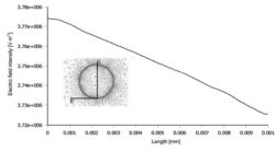
Fig. 6. Distribution of the electric field intensity along the vertical axis of the circular cross-section sample (point 1)
