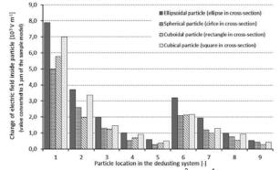
Fig. 8. Change of electric field intensity ( $\cdot 10^3 \text{ V} \cdot \text{m}^{-1}$ ) inside particle for placement in the dedusting system converted to 1  $\mu$ m of the sample model
