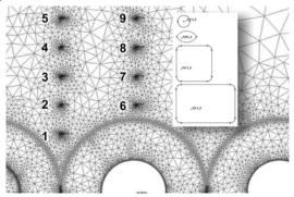
Fig. 5. Placement of dust particles around the bifilar winding during simulation
