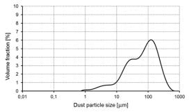
Fig. 2b. Volume distribution of dust particle size for B type dust
