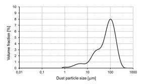
Fig. 2a. Volume distribution of dust particle size for A type dust
