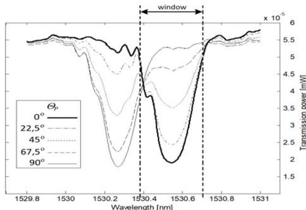
Fig. 3. The typical changes in transmission spectrum of TFBG high order cladding mode influenced by different input light polarization angles
