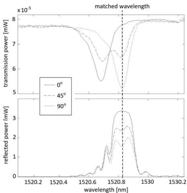
Fig.5. The illustration of measurement idea by showing transmission of cladding mode of TFBG sensor illuminated by light with 3 cases of polarization and reflection response of FBG filter
