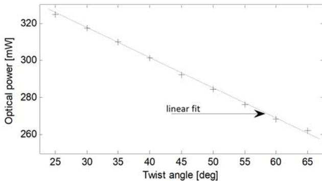
Fig.8. The results of reflected optical power value measured to different twist angles in linear range and best fitting line (dotted line)
