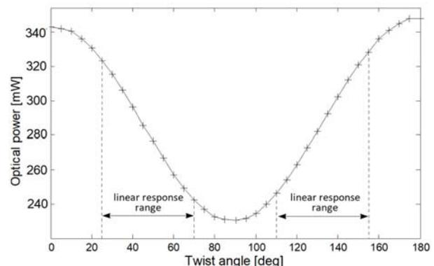
Fig.7. The characteristic of reflected power value changes while twisting of input light polarization angle which illuminates TFBG sensor
