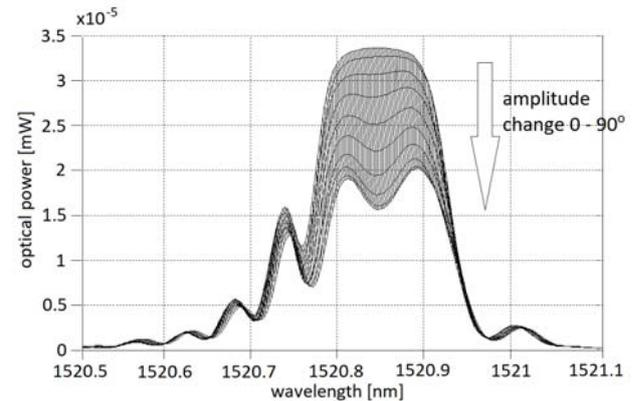
Fig.6. The changes of reflected spectrum of filtering FBG illuminated by transmission of TFBG illuminated with different polarization states of input light
