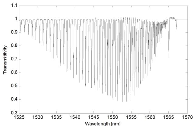
Fig.2. The transmission spectrum of  $6^\circ$  TFBG based twist sensor
