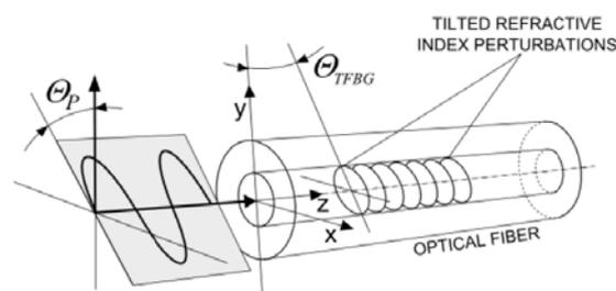
Fig.1. The scheme of TFBG internal structure and angle of input light polarization definition
