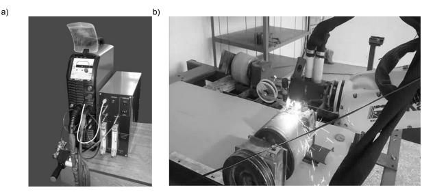
Fig.1. External view of MP-004 manufactured by E. O. Paton EWI, Ukraine (a) and the process of micro-plasma deposition of wire coating on the surface of a cylindrical shaft (b) at the experimental site for micro-plasma surface treatment at D. Serikbayev EKSTU.
