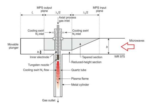
Fig. 1. Draft of the coaxial-line-based nozzleless MPS
