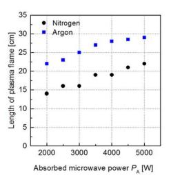
Fig. 5. Influence of absorbed microwave power  $P_A$  on the length of the plasma flame, process gas flow rate Q = 100 l/min
