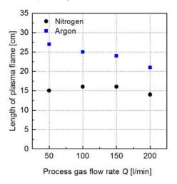
Fig. 6. Influence of process gas flow rate Q on the length of the plasma flame, absorbed microwave power  $P_A$  = 3 kW
