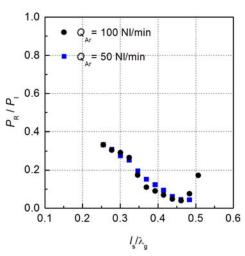
Fig. 4. The MPS tuning characteristics for discharge in argon,  $P_{\rm I}$  = 3 kW
