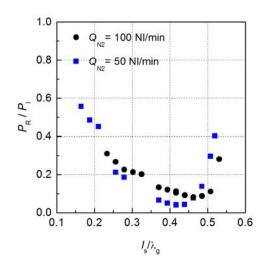
Fig. 3. The MPS tuning characteristics for discharge in nitrogen,  $P_{\rm I}$  = 3 kW
