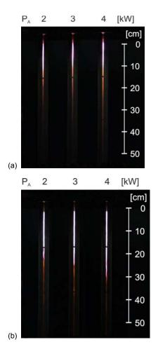
Fig. 7. Photos of microwave discharge in nitrogen (a) and argon (b) for various values of absorbed microwave power  $P_A$ , process gas flow rate Q = 100 l/min
