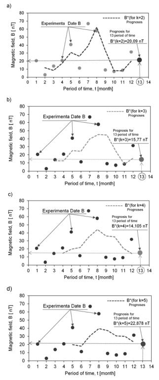
Fig.4 The results of measurements of the induction of magnetic field in the workplace of the operator (DMU 65 Mono Block): a) soothing constant k=2, b) soothing constant k=3, c) soothing constant k=4, d) soothing constant k=5
