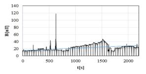
Fig.3. The results of measurements of the induction of magnetic field in the workplace of the operator (DMU 65 Mono Block)
