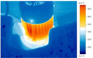
Fig. 4. The motor local overheat detected as a result of heat image control
