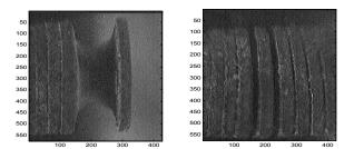
Fig. 1. The stator core teeth zone damage revealed as a result of the video control in the visible and infrared range
