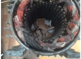
Fig. 2. The stator winding phase-to-phase short circuit detected by the frequency-resonance method
