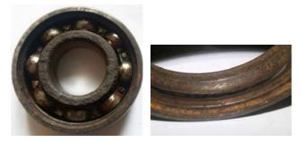
Fig. 3. The presence of the bearing developing damage detected due to vibro-diagnostics
