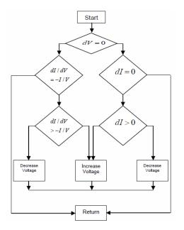
Figure 4: Increment Conductance.
