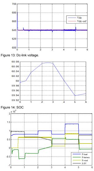
Figure 15: Wind-PV-Battery-Load Hybrid Power
