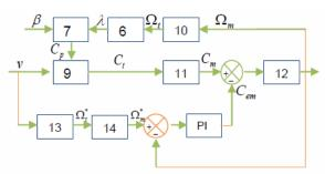
Figure 6: Direct speed control.
