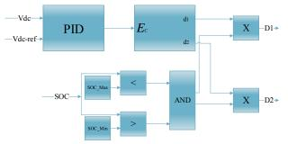
Figure 7: Control of the DC-DC bidirectional converter.
