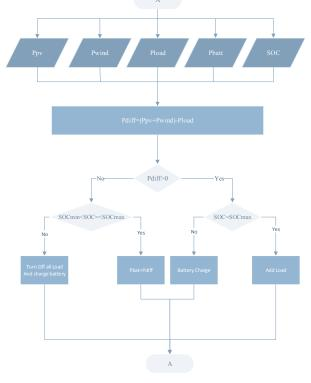
Figure 8: Power management flow chart of hybrid energy system.
