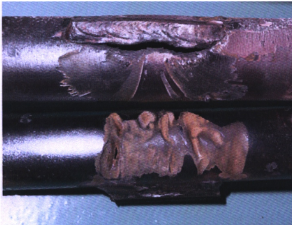
Fig.4. Cracked pipes, damaged on 22nd January 2010. The photo shows two neighboring pipes, which were damaged during that failure. The cracks caused very loud noise in the combustion chamber, what allowed the personnel to detect the fault during routine inspection
