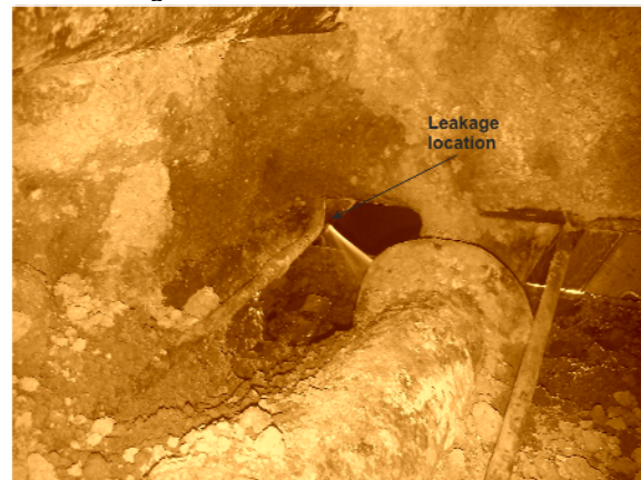
Fig.7. The photograph of the damage, which caused the shutdown of the boiler on 13th January 2014. The leakage occurred in the lower area of the collector chamber; the crack was revealed by the personnel during the routine inspection
