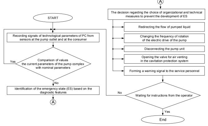
Fig.5. The generalized algorithm of the operation of the system of the diagnostics of unsteady modes of PV operation
