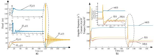
Fig.3. The curves representing the alteration of technological a) and electromechanical (b) parameters of PC at a sharp shutting of the stopcock at time moment *t*=120 s
