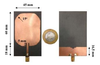
Fig. 1: Built prototype of the multiband antenna.
