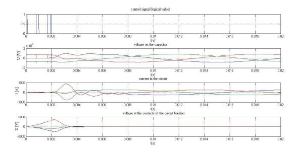
Fig. 12. Waveforms of control signal, voltage on the capacitor, current in the circuit and voltage at the contacts of the vacuum circuit breaker from summary results
