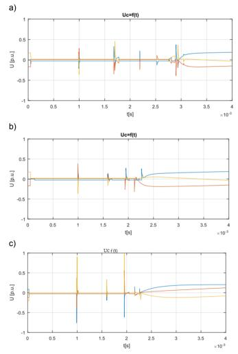
Fig. 11. Waveforms of U<sub>c</sub> voltages on the capacitor clamps. Circuit parameters: bank power Q = 50MVAr, supply voltage Uz = 6kV. Capacitor bank connection systems: a) star b) star with a grounded neutral point c) delta
