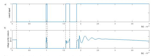
Fig. 8. Influence of the control signal (a) on the voltage at the capacitor clamps (b
