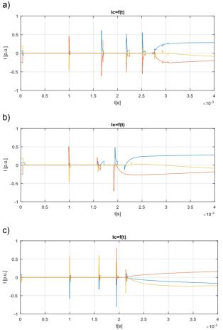
Fig. 10. Waveforms of  $I_c$  current that flows through a capacitor bank. Circuit parameters: bank power Q = 50MVAr, supply voltage Uz = 8kV. Capacitor bank connection systems: a) star b) star with a grounded neutral point c) delta
