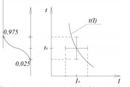
Fig. 2. The time-current characteristic of a fuse and its statistical description of uncertainty for assumed confidence level 0,95
