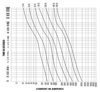
Fig. 1. Sample of a time-current curves for typical time-delay fuse series [2]
