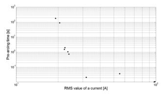
Fig. 3. Time-current characteristic for 6,3 A MV fuses
