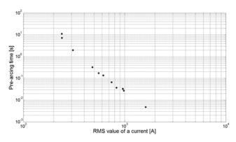
Fig. 4. Time-current characteristic for 63 A MV fuses
