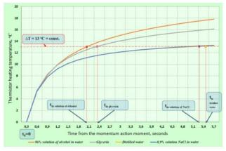
Fig. 7. Method of determining the time of additional thermistor heating to a temperature of  $13^{\circ}$ C in different investigated fluids.
