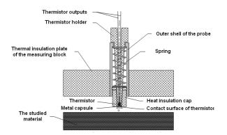
Fig. 2. Location of the thermistor probe and the test substance in studies of solid phase TPC  $% \left( {{{\rm{TPC}}} \right)$
