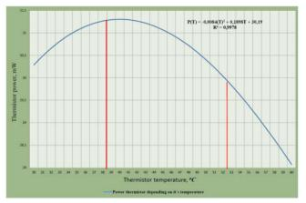
Fig. 5. The dependence of the thermistor's power on it's temperature P=f(t) during the heating (between red vertical lines, the line on the left – the initial heating temperature, the right line – the final heating temperature).
