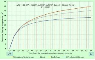
Fig. 4. Thermistor heating thermograms in T=f(t) of various substances (96% solution of ethyl alcohol, glycerol, distilled water, 0.9% NaCl solution in water).
