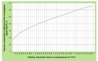
Fig. 8. Measured in the testing process, the real dependence of the value of the thermal conductivity coefficient for studied fluids from the time of thermistor heating to a temperature of  $13^{\circ}$ C.
