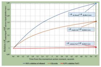
Fig. 6. Measured carried out by the tests, the value of the thermistor heating temperature ratio in the test substances (96% solution of ethyl alcohol, glycerol and 0.9% NaCl solution in distilled water) during the heating pulse.
