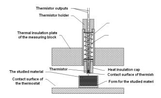
Fig. 3. Location of the thermistor probe and the test substance in TPC studies of conditionally solid and bulk materials [13]
