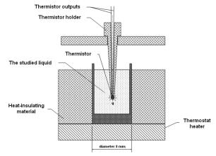
Fig. 1. Location of the thermistor probe and the test in studies of TPC fluids  $% \left( {{\Gamma _{\mathrm{s}}} \right) = {\Gamma _{\mathrm{s}}} \right)$
