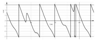
Fig.4. Phase-frequency characteristic of the total signal for three measurement objects with different reflection coefficients
