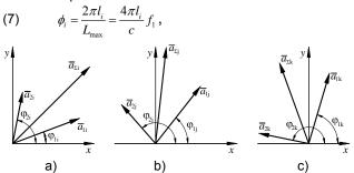
Fig. 2 Vector diagrams of signals reflected from two objects and the total signal on the i-th (a), j-th (b) and k-th (in) frequencies
