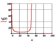
Fig.5d. Dependence of the time of permanence on buffer  $t_b$  from the performance of the block  $p_n$  and the productivities of the general block  $u_n$ =55
