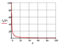
Fig.5a. Dependence of the operating time of the  $t_n$  block on the productivity of the block to the amount of the raw material by the block r=50
