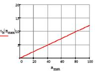
Fig.5c. Dependence of the time of permanence on buffer size for the performance of the block p=45 and the productivities of the general block  $u_n$ =55
