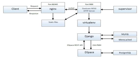
Fig.2. The scheme of interaction of the Academgorodok portal with the components of a distributed information system
