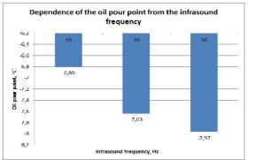
Fig.2. The diagram of dependence of the oil pour point on the infrasound frequency
