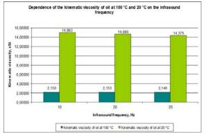
Fig.4. The diagram of the dependence of the kinematic viscosity of oil at 100  $^\circ\text{C}$  and 20  $^\circ\text{C}$  on the infrasound frequency
