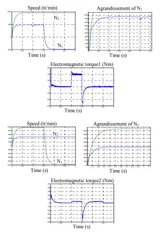
Fig .10. Test of robustness of the fuzzy regulator with applied load torque and the change of rotation direction during a variation of the moment of inertia (J =  $2J_n$ ) for M(1) and (J<sub>2</sub>= $2J_{n2}$ ) for M (2).
