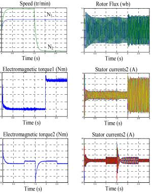
Fig .9. Performance of indirect vector controlled system: The I.M(2) reverses from +100 to -100 rad/s using fuzzy controller
