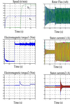
Fig .7. Performance of indirect vector controlled system: Acceleration of I.M(1) from 0 to 50 rpm using fuzzy controller
