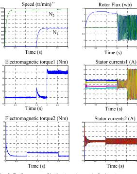
Fig .6. Performance of indirect vector controlled system: Acceleration of I.M(2) from 0 to 100 rad/s using fuzzy controller
