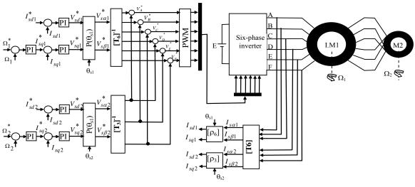
Fig. 2. Indirect rotor flux oriented controller for the two-motor drive
