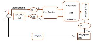
Fig. 3. Block diagram of fuzzy controller
