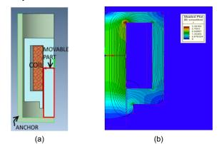
Fig.11. Electromagnetic actuator: cross-section (a), magnetic flux lines (b).
