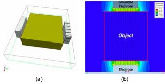
Fig.10. Capacitive sensor: 3D geometry (a), electric field map (b).
