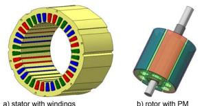
a) stator with windings b) rotor with PM Fig.5. Permanent magnet synchronous motor assembling parts
