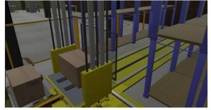
Fig.7. Pulling off the package from roller conveyor to lift platform
