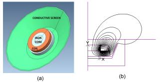
Fig.9. Inductive sensor: 3D geometry (a), magnetic flux lines (b).
