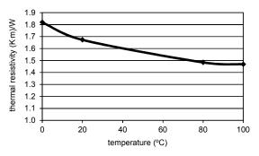
Fig.10. Thermal resistivity of water (pressure 1  $\mbox{kg/cm}^2)$  as a function of its temperature [20]
