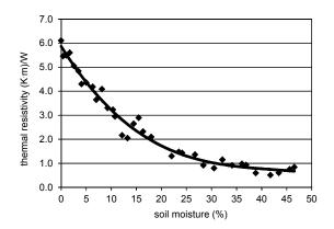
Fig.4. Thermal resistivity of the top layer of soil with organic particles, as a function of its moisture (weight moisture)
