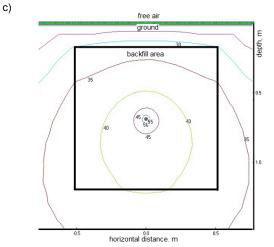
Fig.8. Temperature distribution (°C) around a power cable YKY 1×240 mm<sup>2</sup> (depth 0.7 m, initial temp. 20°C, max temp. 70°C) for thermal resistivity of the native soil  $\rho_{\rm soil}$  = 2.5 (K m)/W, stabilized backfill  $\rho_{\text{back}}$  = 0.5 (K·m)/W and its dimensions:
