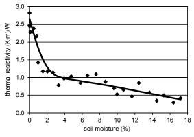
Fig.5. Thermal resistivity of sand (fraction ≤2 mm) as a function of its moisture (weight moisture)
