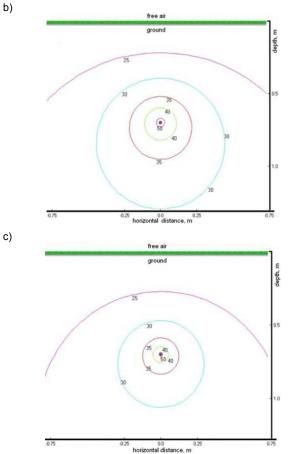
Fig.7. Temperature distribution (°C) around a power cable YKY 1×240 mm2 (depth 0.7 m, initial temp. 20°C, max temp. 70°C) for thermal resistivity of the soil: a)  $\rho_{\rm soil}$  = 2.5 (K·m)/W,  $I_z$  = 507 A, b)  $\rho_{\text{soil}}$  = 1.0 (Km)/W,  $I_z$  = 732 A, c)  $\rho_{\text{soil}}$  = 0.5 (Km)/W,  $I_z$  = 916 A
