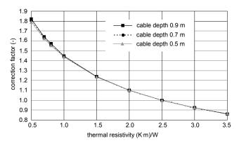
Fig.2. Correction factors of the current-carrying capacity calculated according to IEC 60287 [12, 13], for a cable YKY 1×240 mm<sup>2</sup> (copper conductor, PVC insulation and sheath) directly buried in the ground, for various thermal resistivities of the soil and cable depth. Reference thermal resistivity of the soil: 2.5 (Km)/W
