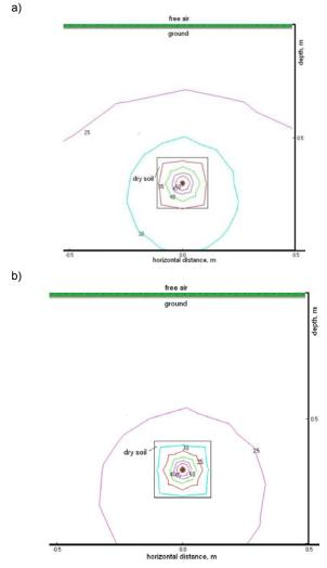
Fig.9. Temperature distribution (°C) around a power cable YKY 1×240 mm<sup>2</sup> (depth 0.7 m, initial temp. 20°C, max temp. 70°C), taking into account the drying of the soil with the cable load; thermal resistivity of the dry soil near the cable (10 cm horizontally and vertically from cable surface) is 2.5 (Km)/W. Thermal resistivity of the native soil is: a) 1.0 (K m)/W,  $I_z = 614$  A, b) 0.5 (K m)/W,  $I_z = 660 \text{ A}$
