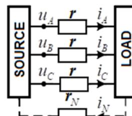
Fig. 1. Three-phase power supply system with resistive model of the transmission line
