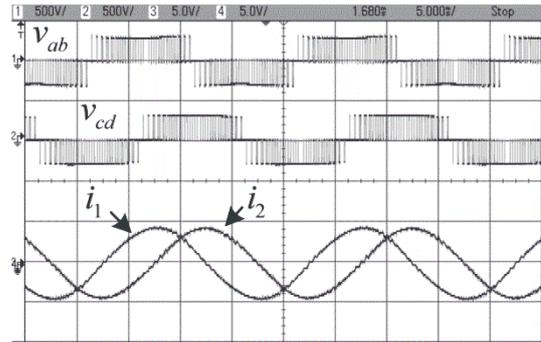
Fig. 12. Output voltage  $v_{ab}$  and  $v_{cd}$ , output current  $i_1$  and  $i_2$  of CSVPWM.
