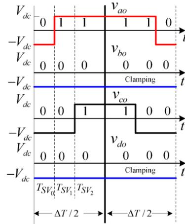
Fig. 4. Pulse pattern and phase-leg reference voltage for the sector 1
