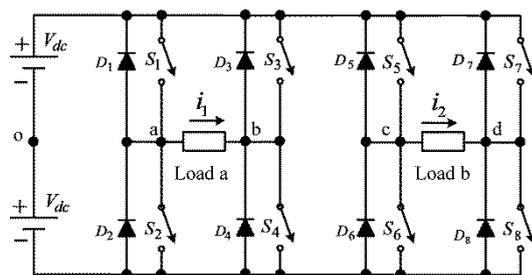
Fig. 1. A proposed two-phase four-leg voltage source inverter
