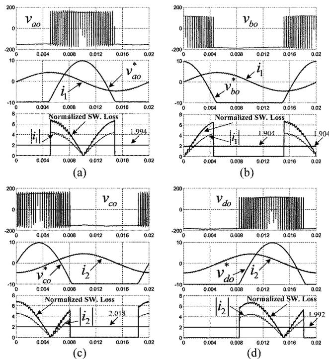
Fig. 15. Normalized switching losses of proposed DSVPM in each phase-leg.
