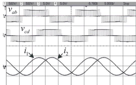
Fig. 13. Output voltage  $v_{ab}$  and  $v_{cd}$ , output current  $i_1$  and  $i_2$  of DSVPWM.
