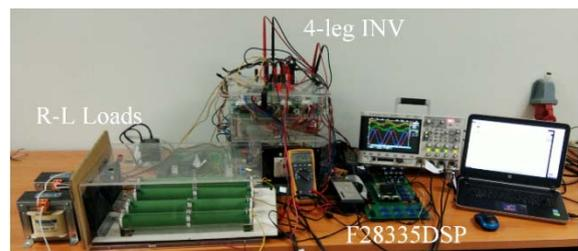
Fig. 8. Experimental setup for two-phase four-leg VSI system
