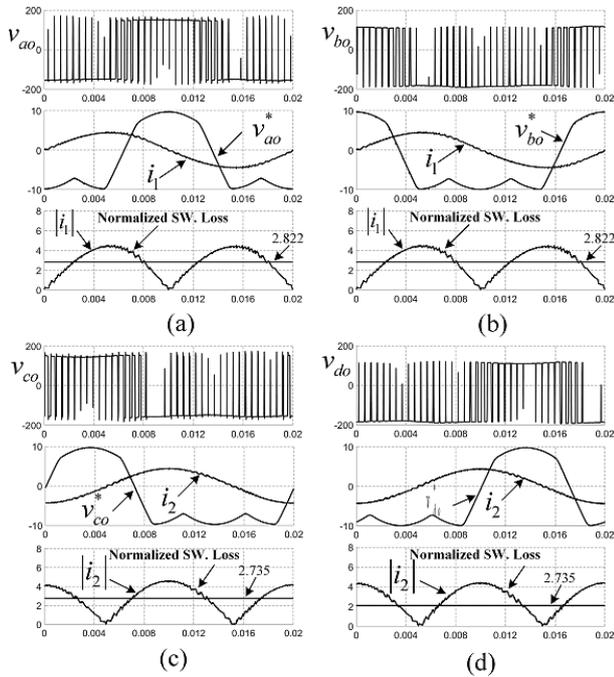
Fig. 14. Normalized switching losses of CSVPWM in each phase-leg.
