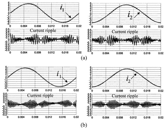
Fig. 16. Measured load current ripple (a) CSVPWM and (b) proposed DSVPM
