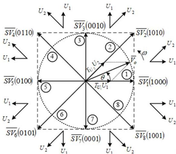
Fig. 2. Location of active space vectors in d-q plane and arbitrary output voltage.
