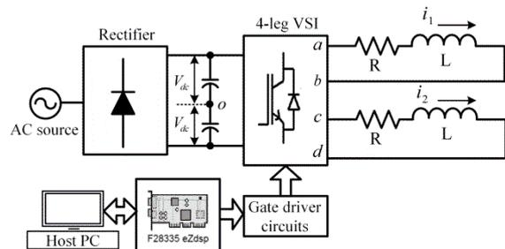
Fig. 7. A proposed two-phase four-leg VSI system
