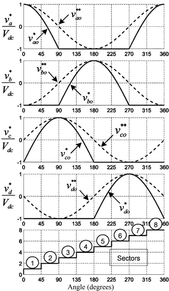
Fig. 5. Phase-leg reference voltage waveforms for proposed DSVPWM
