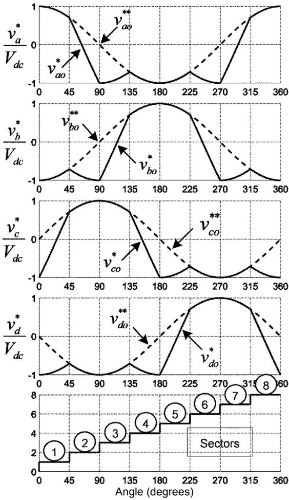
Fig. 3. Phase-leg reference voltage waveforms for CSVPWM
