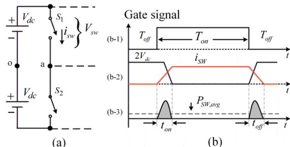
Fig. 6. Switching loss characteristics (a) one-leg inverter power circuit (b) Linearized switching characteristics (b-1) gate driver signal (b-2) voltage cross switching and load current flowing through switching device S<sub>1</sub> (b-3) average switching power loss.
