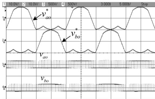
Fig. 10. CSVPWM (a) four phase-leg reference voltage of  $v_{ao}^*$ ,  $v_{bo}^*$  and output phase voltage of  $v_{ao}$ ,  $v_{bo}$ .
