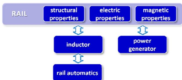
Fig.3. Concept of an energy-efficient induction heating system of railway turnouts
