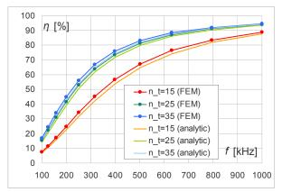
Fig.8. Results comparison of power transfer efficiency dependent of number of turns  $(n_t)$  for the case h = 5 mm
