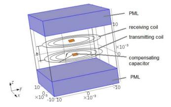
Fig.3. A three-dimensional view on one of WPT cell
