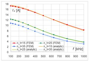
Fig.5. Results comparison of source current  $(I_z)$  dependent of number of turns  $(n_t)$  for the case h = 10 mm
