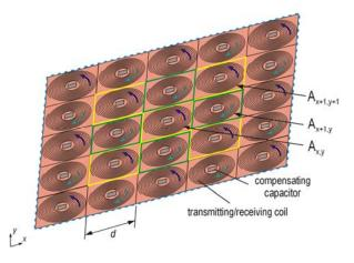
Fig.2. A two-dimensional network transmitting/receiving surface of the non-periodic WPT system ( $A_{x,y}$  – the WPT cell)
