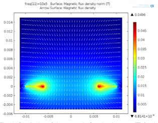
Fig.11. Distribution of the magnetic flux density norm [T] for the case  $n_t = 15$ , h = 10 mm (XZ plane)
