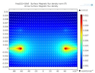
Fig.10. Distribution of the magnetic flux density norm [T] for the case where the number of turn is 15, h = 5 mm (XZ plane)
