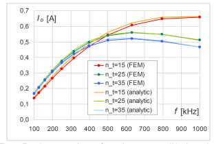
Fig.7. Results comparison of receiver current ( $I_o$ ) dependent of number of turns ( $n_t$ ) for the case h = 10 mm
