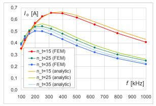
Fig.6. Results comparison of receiver current  $(I_o)$  dependent of number of turns  $(n_t)$  for the case h = 5 mm
