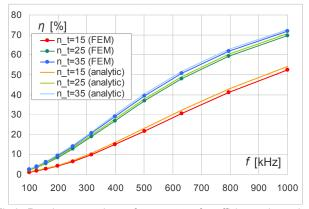
Fig.9. Results comparison of power transfer efficiency dependent of number of turns  $(n_t)$  for the case h = 10 mm
