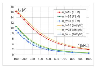
Fig.4. Results comparison of source current  $(I_z)$  dependent of number of turns  $(n_t)$  for the case h = 5 mm
