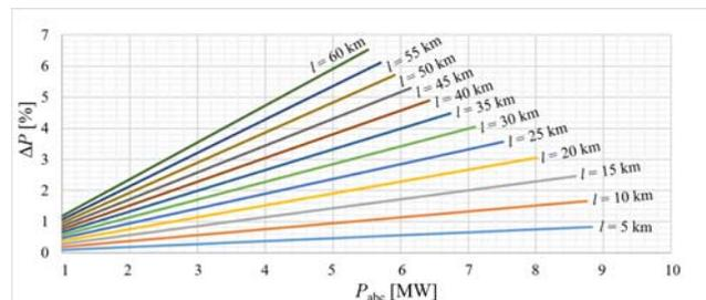
Fig.3. The active power losses for NA2XS2Y 240/25
