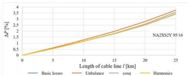
Fig.20. Active power losses on MV side for Location 10
