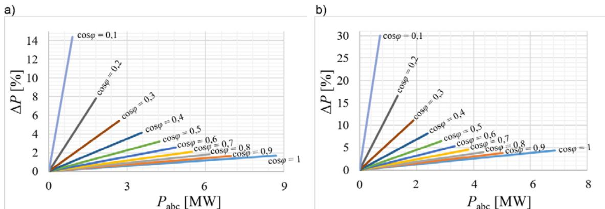
Fig.12. The active power losses for NA2XS2Y 240/25: a) the length of 10 km, b) the length of 30 km
