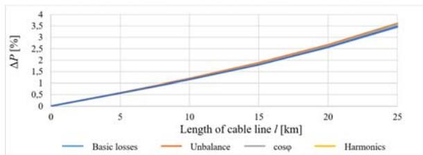
Fig.19. Active power losses on MV side for Location 5
