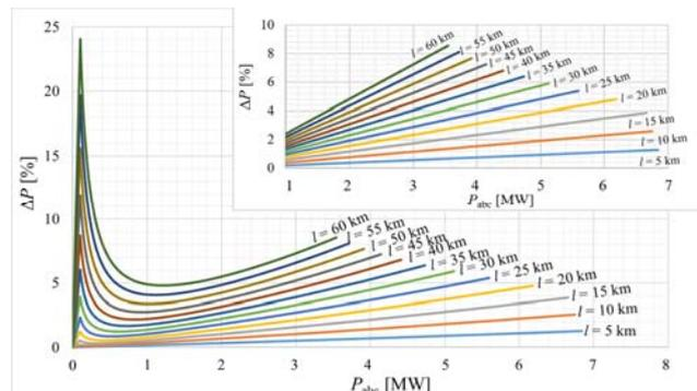
Fig.2. The active power losses for NA2XS2Y 150/25
