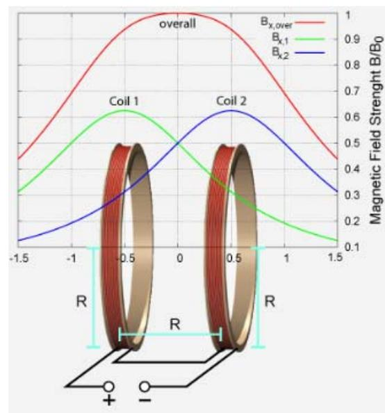
Fig. 1. Helmholtz coil and its magnetic field [3,4]
