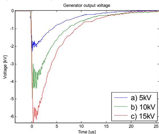
Fig.4. The Voltage produced by Marx generator in three ranges: 5 kV, 10 kV and 15 kV.
