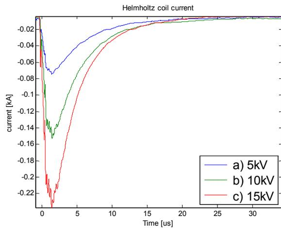
Fig.5. Current flowing through the Helmholtz coil, measured at 5 kV, 10 kV and 15 kV, using Rogowski coil with Rogowski current waveform transducer CWT 60B.
