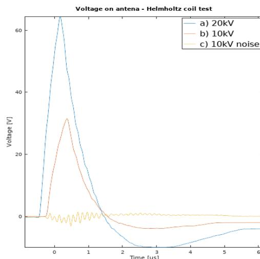
Fig.7. The disturbances induced in measuring lines at 10 kV (20 kV for comparison).
