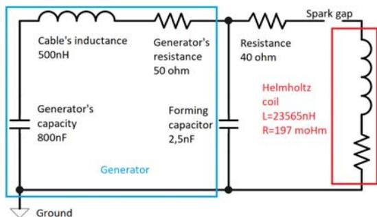
Fig.3. Simplified system for uniform magnetic field of lightning-like electromagnetic pulse.
