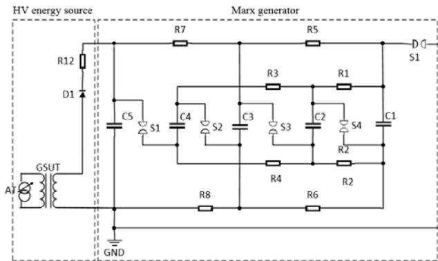
Fig.2. The Marx generator diagram.
