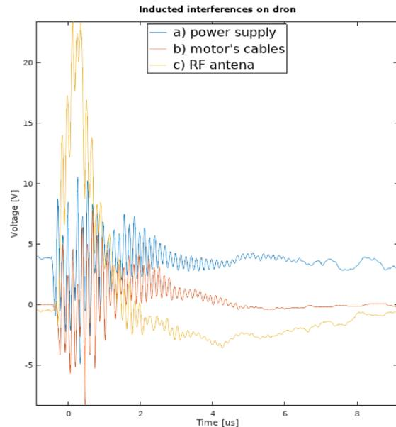
Fig. 9. Induced interference in selected, critical elements of the drone.
