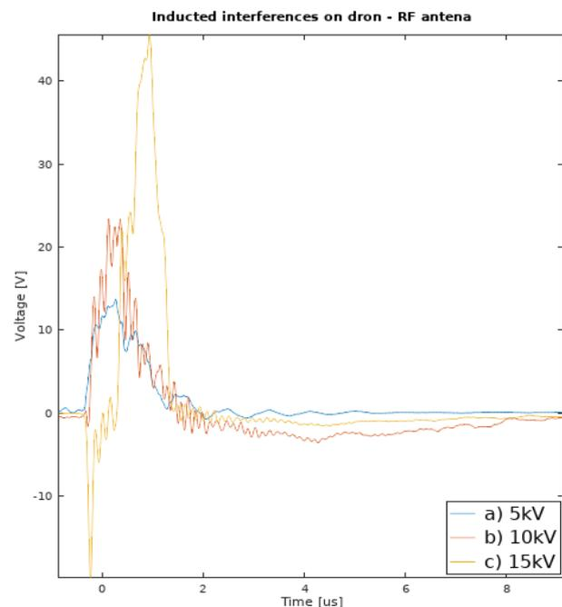
Fig. 10. Disturbance Induced in RF antenna at excitation voltage:  $5\ \text{kV}$ ,  $10\ \text{kV}$  and  $15\ \text{kV}$ .
