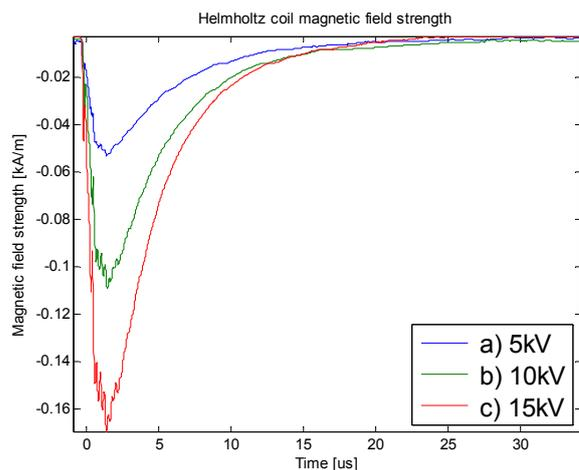
Fig.6. Intensity of the magnetic field in the centre of the Helmholtz coil at 5 kV, 10 kV and 15 kV.
