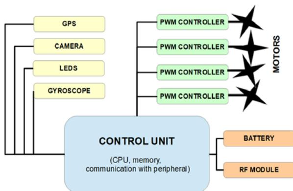
Fig. 8. Block diagram showing the most important elements of the drone.
