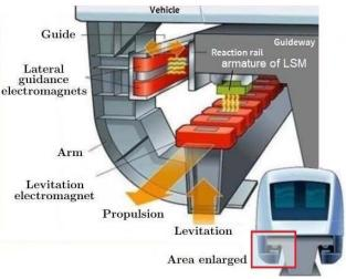
Fig. 3. Principle of operation of Transrapid maglev system.
