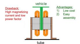
Fig. 15. Double-side LIM with aluminum secondary (reaction rail)
