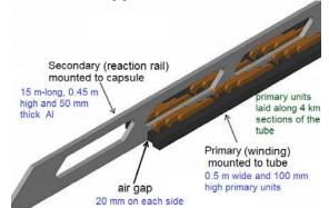
Fig. 10. Double-sided LIM for propulsion according to E. Musk [6]
