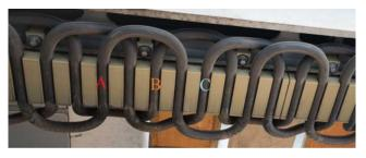
Fig. 4. Track-mounted armature winding of LSM made of aluminum power cable. There are single-turn coils with full-pitch coil span.
