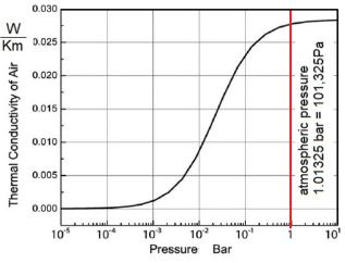
Fig. 17. Thermal conductivity of air as a function of pressure.
