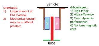
Fig. 16. Double-sided PM LSM with coreless primary (armature)
